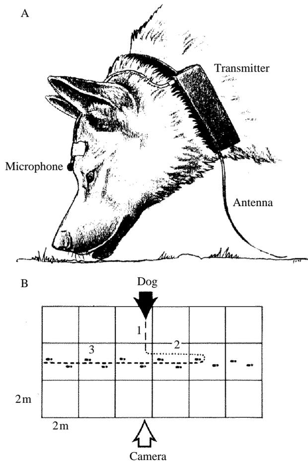
Fig. 1. (A) The position of the microphone and transmitter while the dog was tracking. (B) How the footprints were placed in the 2 m $\times$ 2 m grid, and one example of a dog's path during the searching phase (1), the deciding phase (2) and the tracking phase (3). Only 18 of the 40 squares are shown.
